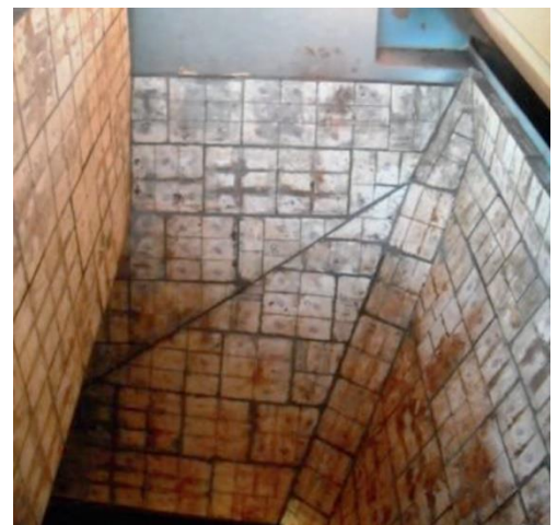
CorroTile™ liners installed in a reclaimer chute
